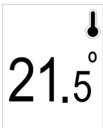
The screen will change to show the current room temperature. You can now set the temperature required with the **▼** and **▲** keys and turn the heater on and off with the **ON/OFF** button. None of the other keys or functions are available.
