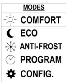
In normal operation mode touch the **MODE** button and the screen will change to show the Modes Menu. Touch the **▼** button until **CONFIG** is highlighted and touch **OK**,
